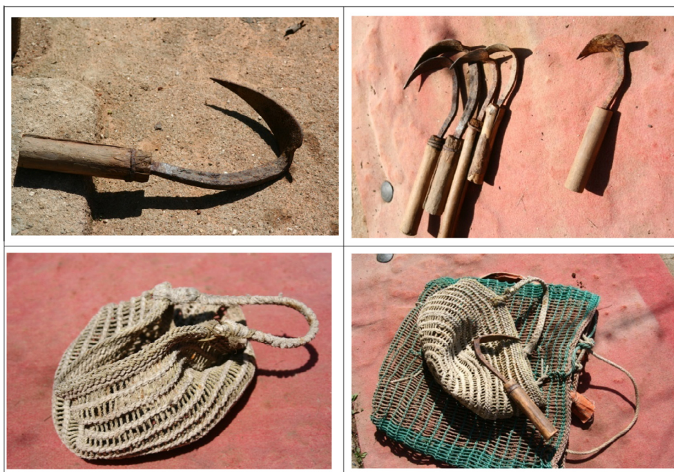
Fig. 4 Fishing gears used for manila clam collection on tidal flats. Top-left: manila clam hand hoe, top-right: fishing hand hoes and farming hand hoe (right), bottom-left: jongtaegi (carrying mesh basket), bottom-right: jongtaegi and mangtaegi (carrying mesh rucksack).
